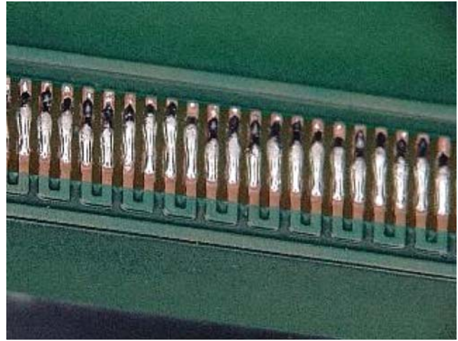
Figure 1-4 Open or Insufficient Solder Joints
